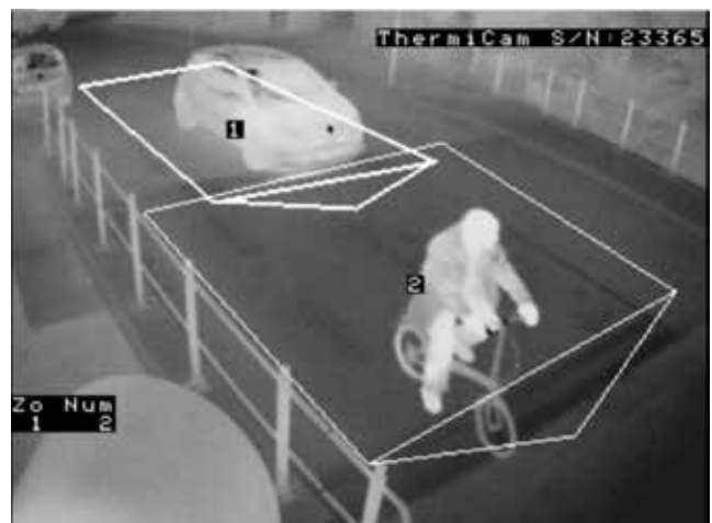
A dedicated bicycle traffic signal scheme based on thermal imaging sensors from FLIR Systems in the city of Utrecht, the Netherlands
